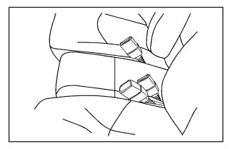
Your vehicle may have a front center seat. There are cupholders on the underside of the seat cushion. To use them, flip the seat cushion forward. This seat can also be used as a storage area by lowering the seatback. See *Center Console Storage Area on page 143*. The seatback doubles as an armrest for the driver or front passenger when the center seat is unoccupied.
